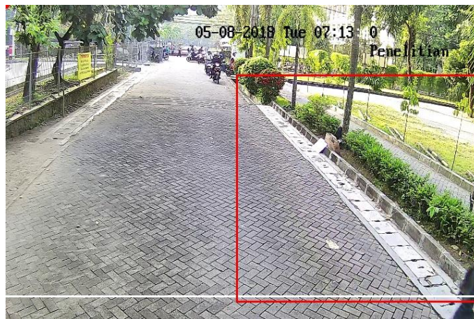
Figure 10. MoG2 Background Substruction with Sobel x, Threshold, Closing, Erosion, Dilation, and Contours
