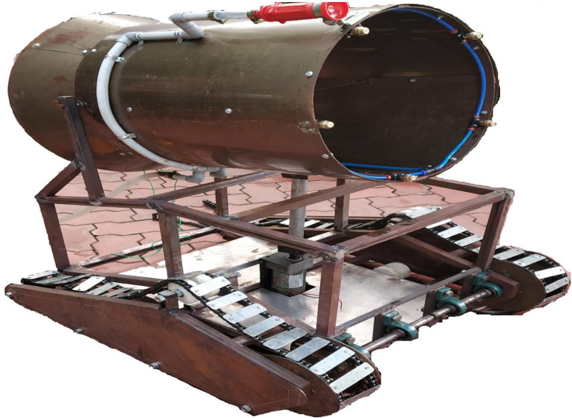
Fig.6. Prototype Model of Rover X model for autonomous control
