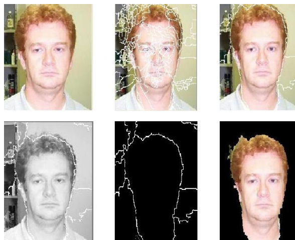
(d) (e) (f) Fig.6 (a) Input Image, (b) Initial Segmented Image, (c) Merged Image using region merging (after 5th iteration) (d) Grey-scale Image (e) Image mask (f) Desired portion of Image
