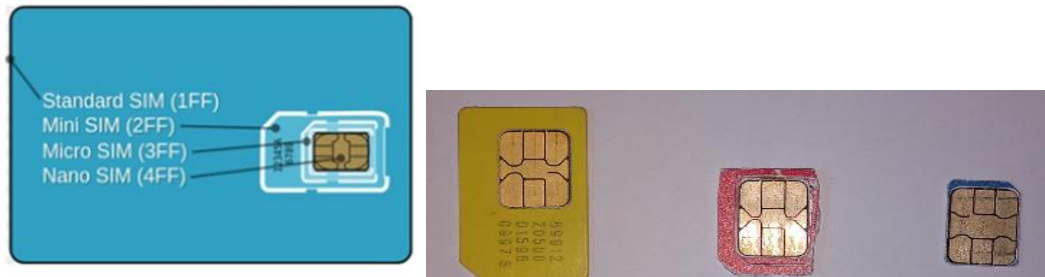
Figure 1(a): Shape of SIM card Figure 1(b): Sizes of Mini, Micro, Nano SIM cards
