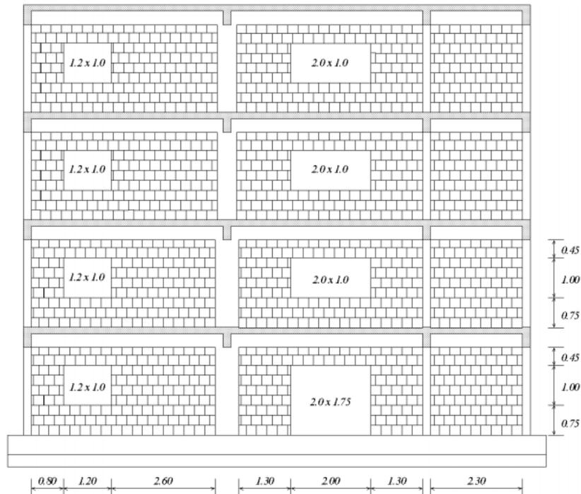
Fig. 1 Four-storey 2D infilled frame (ICONS frame) [3]
