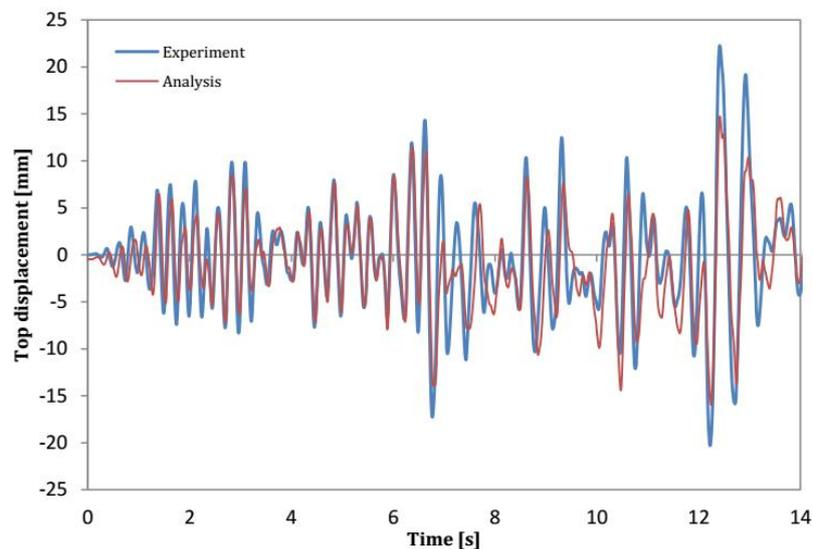
Fig. 2 Experimental vs. Analytical results – top displacement-time (975yrp) [4]
