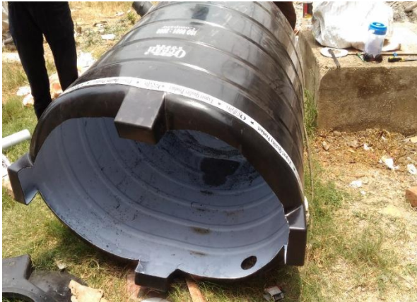
Fig 4. Digester tank of 1000 litres
