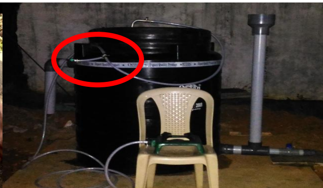
Fig.10 Moisture trap system
