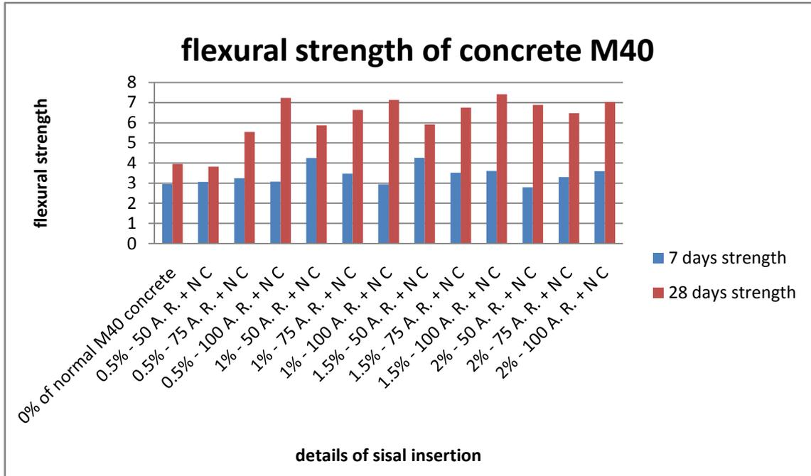
Flexural strength of concrete for M40 mix
