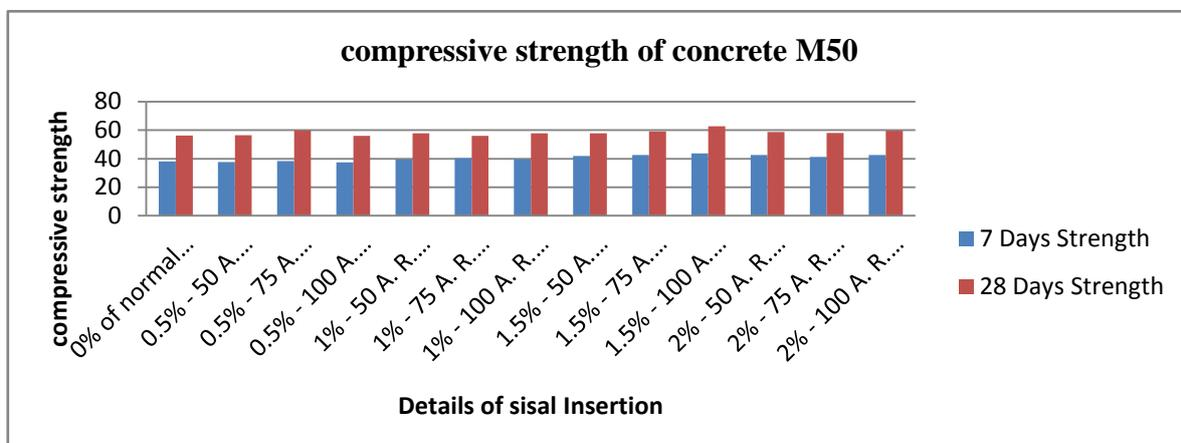
**Compressive strength of concrete for M50 mix**
