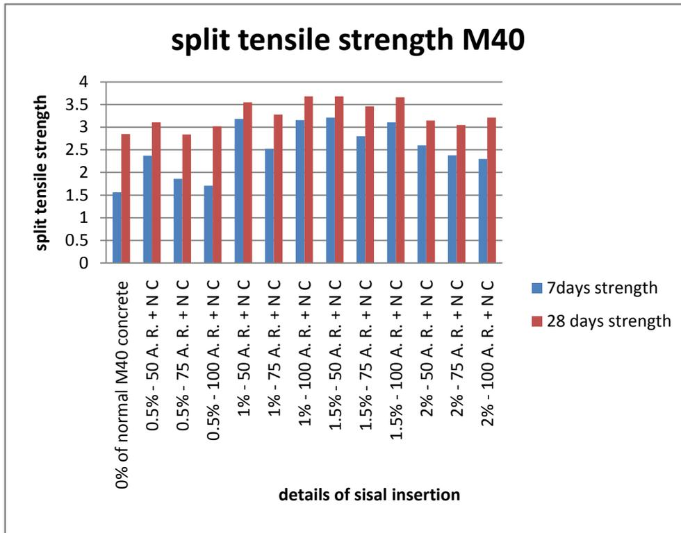
Split tensile strength of concrete for M40 mix
