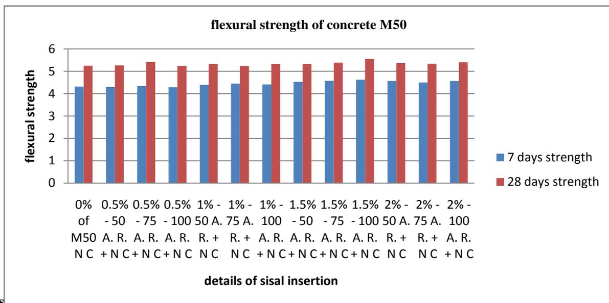
Flexural strength of concrete for M50 mix
