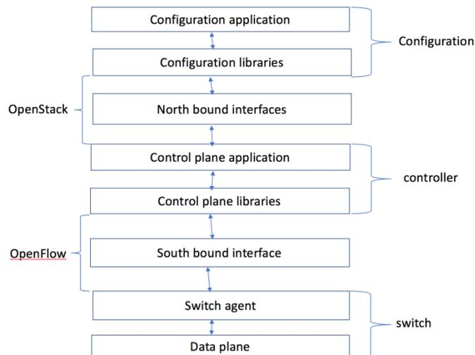
Figure 6. Layers in SDN Architecture
