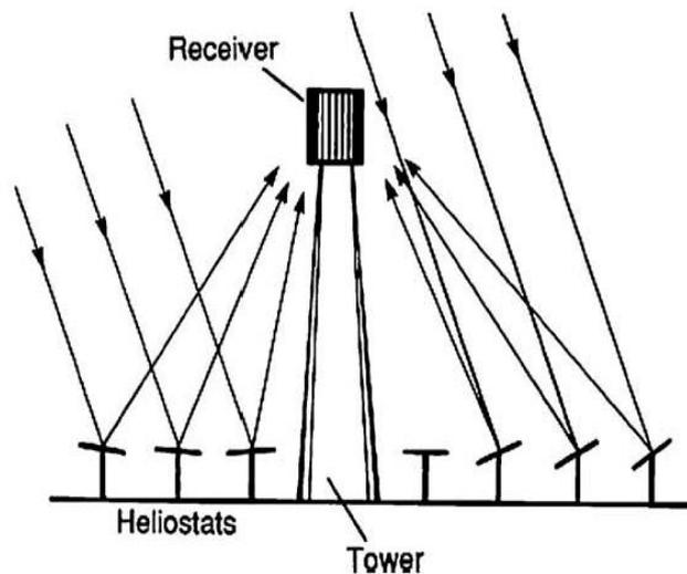
**Fig. 1.** Parabolic trough system **Fig.2.** Central Receiver Tower System
