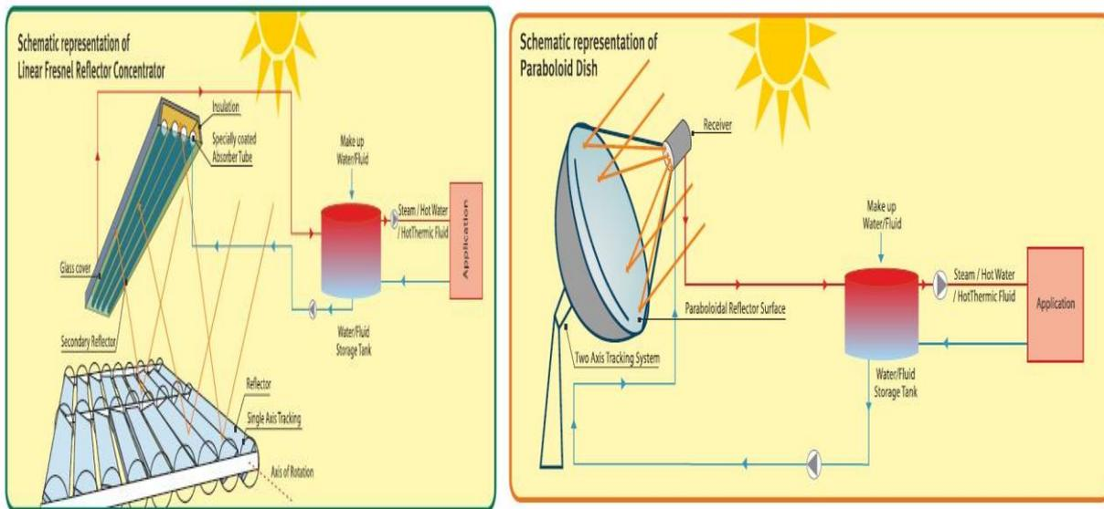
**Fig. 3.** Schematic representation of Linear Fresnel Reflector Concentrator [9] **Fig. 4.** Schematic representation of Parabolic Dish Reflector [8].
