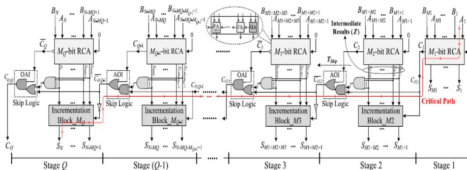
Fig 2. Proposed structure of CSKA
