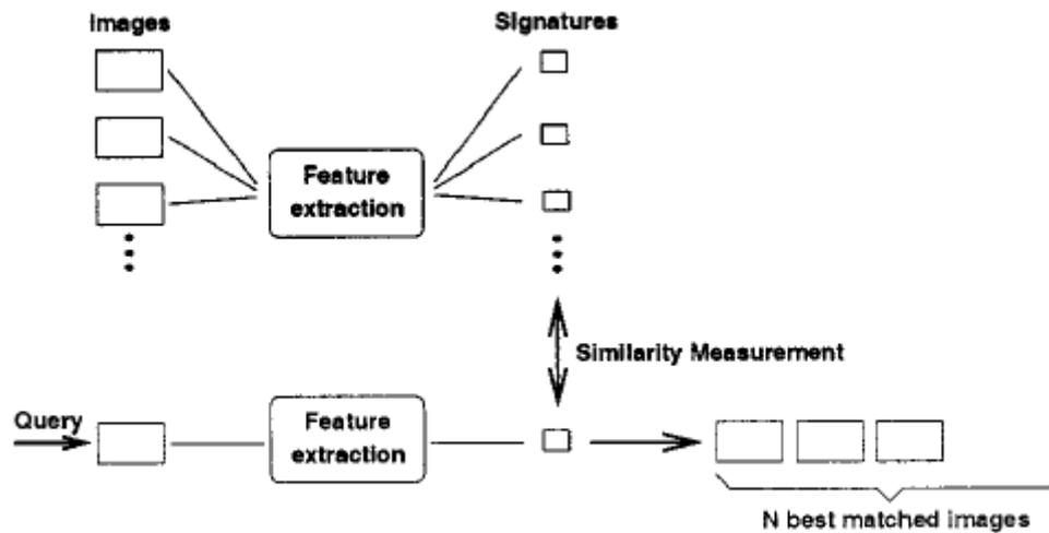
Fig. 1. Image retrieval system architecture.
