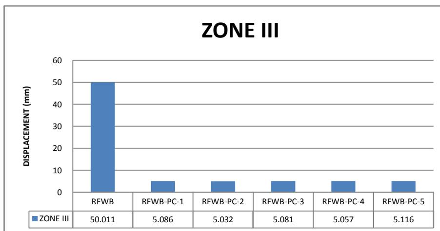
Comparison of displacements for seismic zone III
