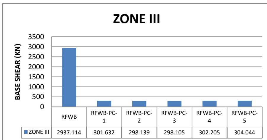
Comparison of base shear for seismic zone III
