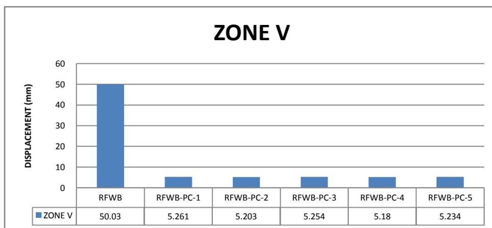
Comparison of displacement for seismic zone V
