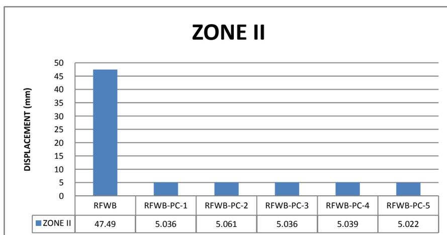
Comparison of displacements for seismic zone II
