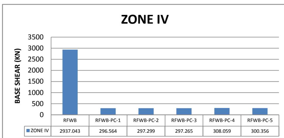
Comparison of base shear for seismic zone IV
