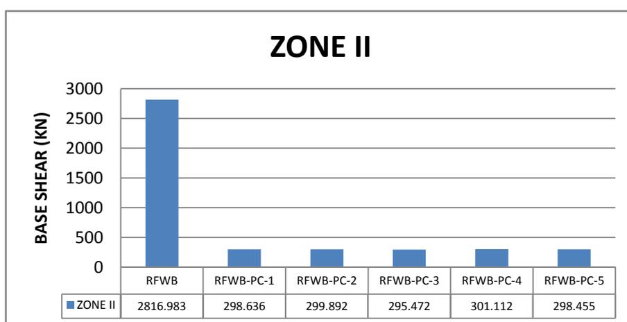
Comparison of base shear for seismic zone II
