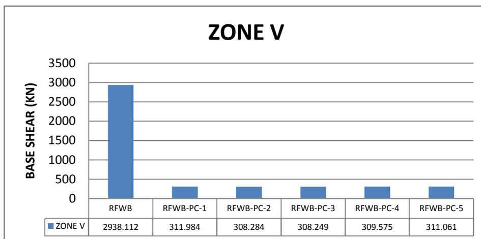
Comparison of base shear for seismic zone V
