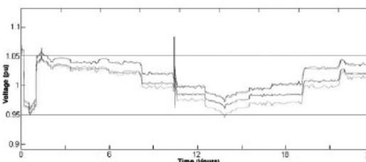
Fig.4.Voltage of the proposed system after regulation
