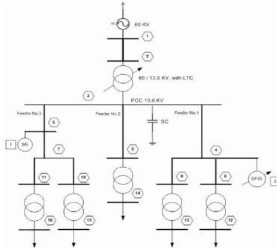
Fig.2. Proposed 16-bus system with DGs
