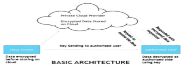
Fig 4. Basic Architecture Showing Encryption and Decryption Process
