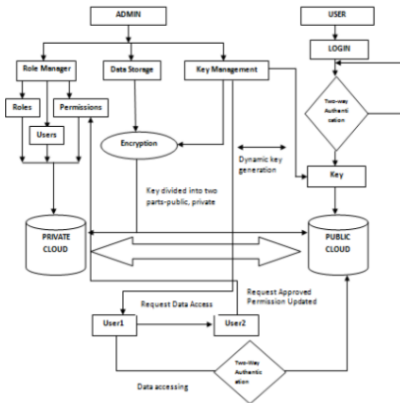
Fig. 2 Secure Data Sharing in Cloud Computing using Hybrid cloud
