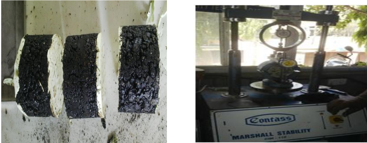
Fig. 5.3 Marshal Stability Test specimens & its testing
