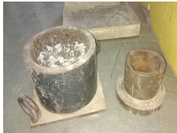
Fig. 5.2 Aggregate crushing value test apparatus
