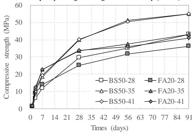
Fig. 1 Test results for compressive strength
