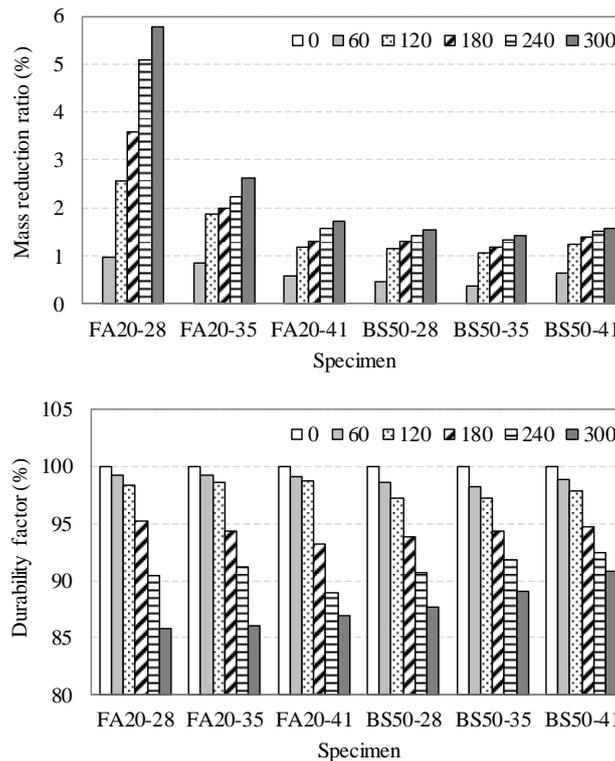
(a) Mass reduction ratio of freezing and thawing
