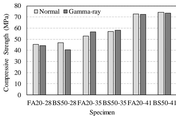
**Fig. 4 Effects of gamma-ray radiation on concrete strength**
