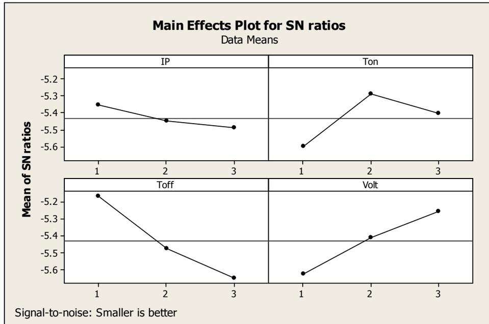
Figure 2 S/N ratio for Surface Roughness
