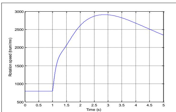
Fig.11. Rotation speed, Nf ≈ 2800 trun/mn
