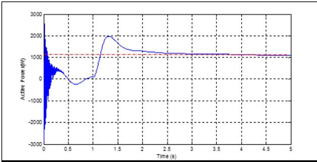
Fig. 4. Active power, final value  $P_f \approx 1100W$
