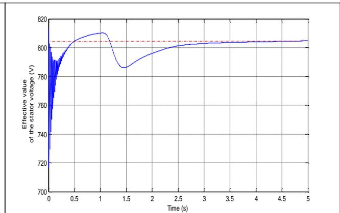
Fig.7. Effective value of the stator voltage (V)  $U_{fs} \approx 804V$
