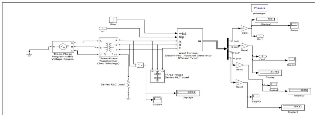
Fig.8. Block diagram of a Wind Turbine driven by a Doubly-Fed Induction Generator
