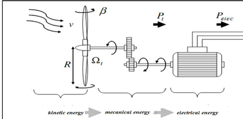
Fig.1.Schematic of a general wind chain
