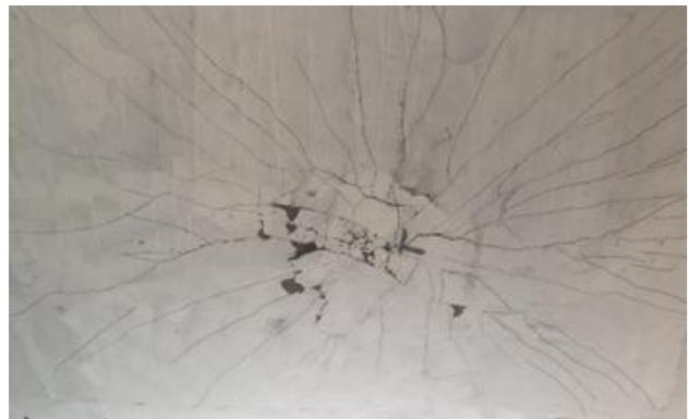
Fig. 10 Failure pattern of specimen
