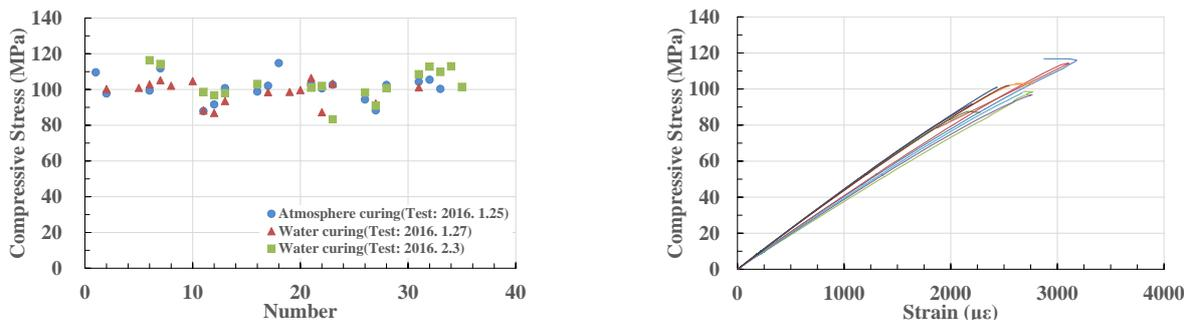
Fig. 9 Experimental compressive strength and elastic modulus of SC-100
