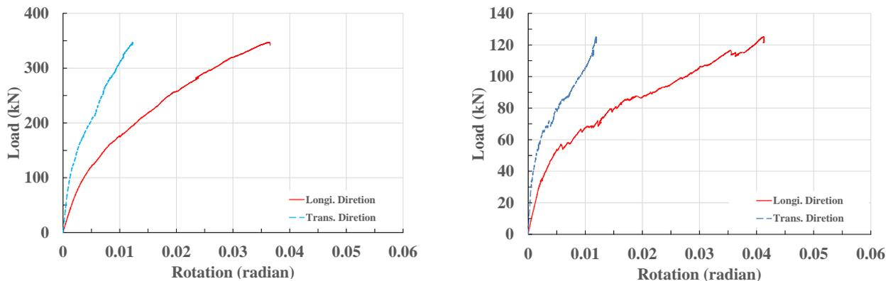
Fig. 12 Experimental end angle rotation of deck
