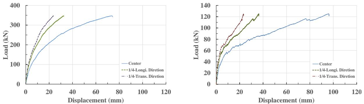
Fig. 11 Experimental deflection of deck
