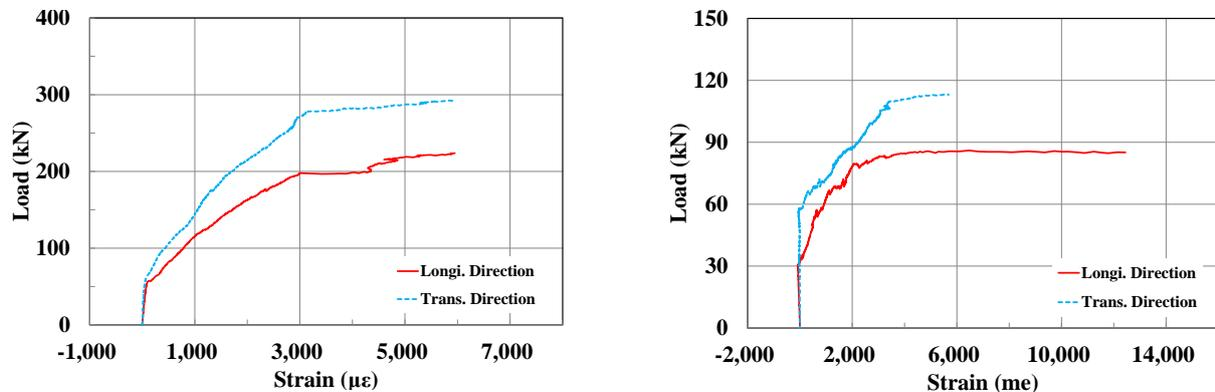
Fig. 13 Experimental strain at centre of deck
