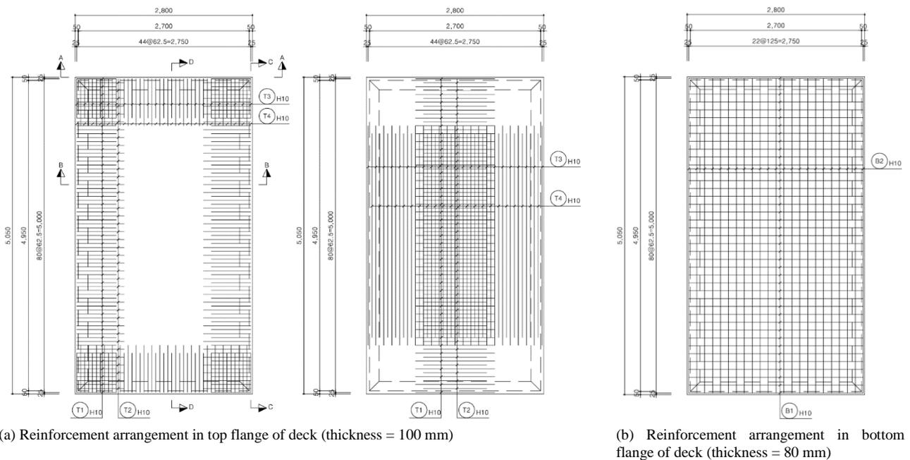
Fig. 6 Arrangement of reinforcement at top and bottom flanges of deck specimen
