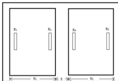
Fig.3.5 Piezoresistor placement on the optimized single boss diaphragm ‘C7’
