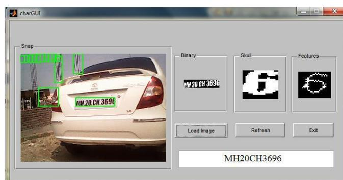
Figure 12. GUI model for license plate recognition system
