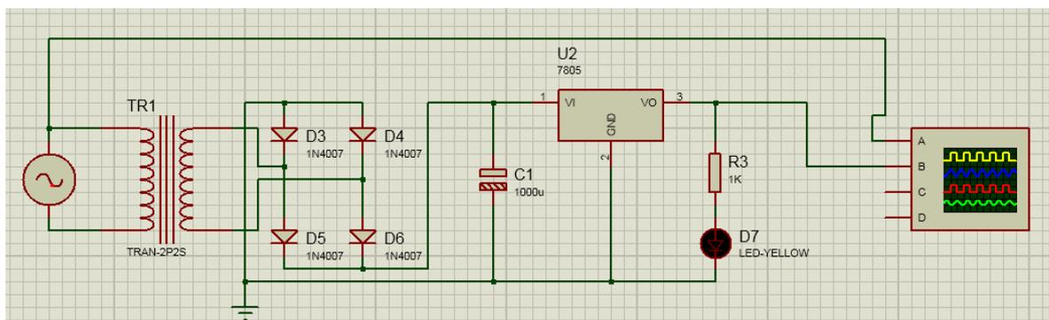
Figure 2. Circuit diagram for Power supply
