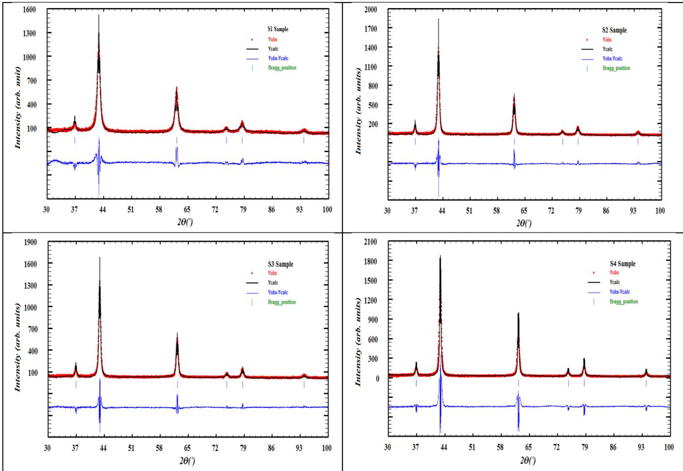
Fig. 3. Rietveld refinements of MgO-NPs for S1, S2, S3 and S4 samples.
