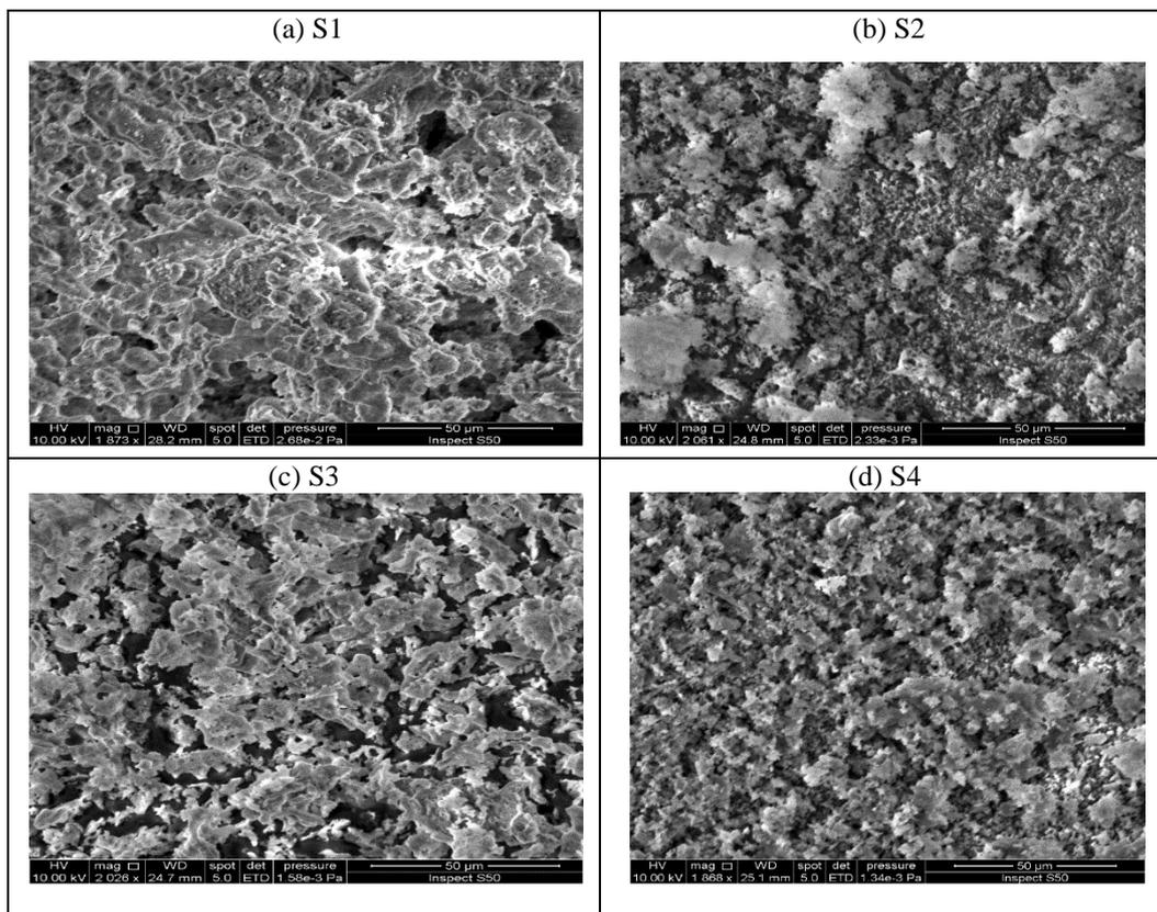
**Fig. 4.** SEM images of MgO-NPs
