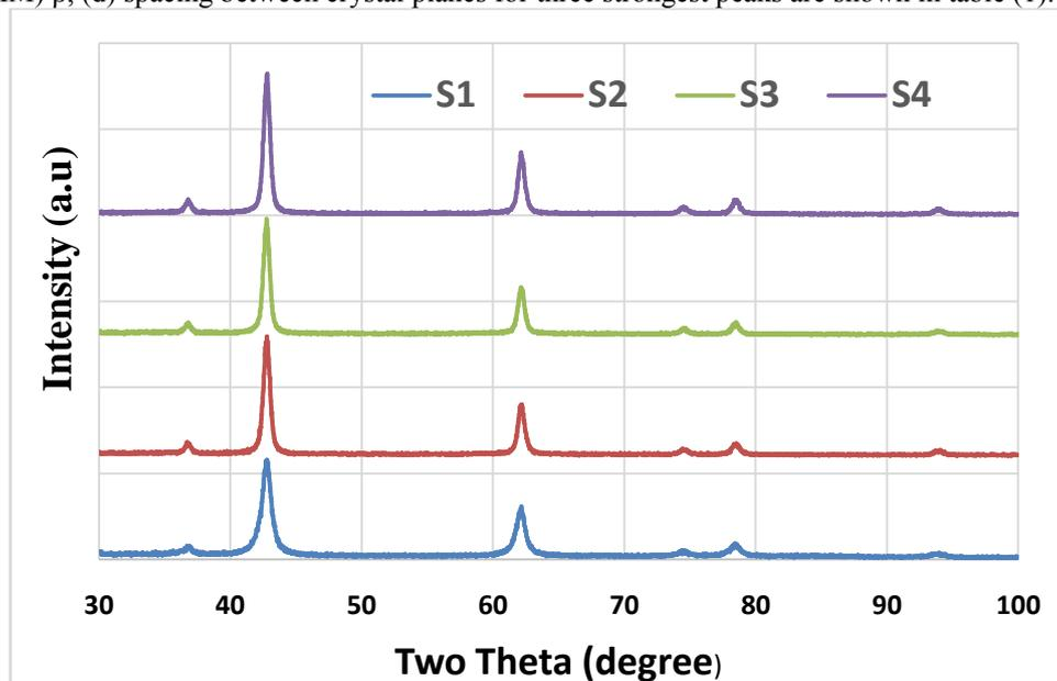
Fig. 1. XRD pattern of MgO-NPs
