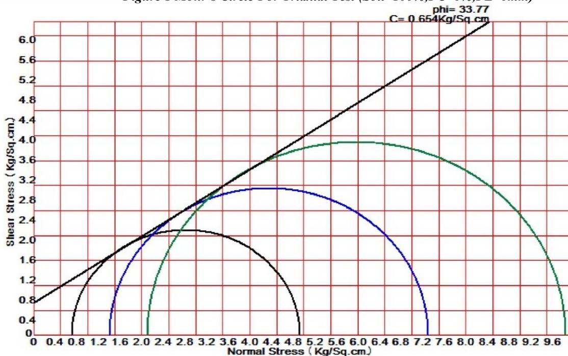
*Figure 2 Mohr's Circle For Triaxial Test (Soil=100%,FC=0.1%,FL=6mm)*
