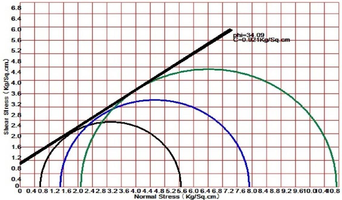
Figure 4 Mohr's Circle For Triaxial Test (Soil=100%,FC=0.3%,FL=6mm)
