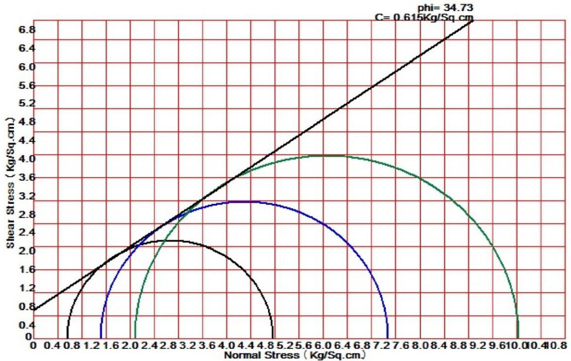
Figure 3 Mohr's Circle For Triaxial Test (Soil=100%,FC=0.2%,FL=6mm)
