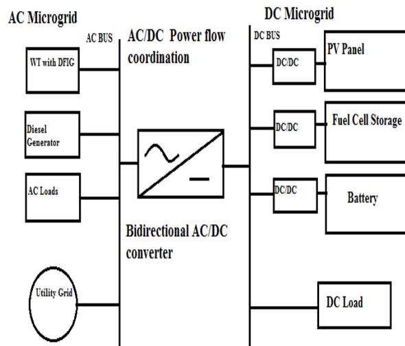
FIG3:Schematic diagram of hybrid AC/DC micro-grid.
