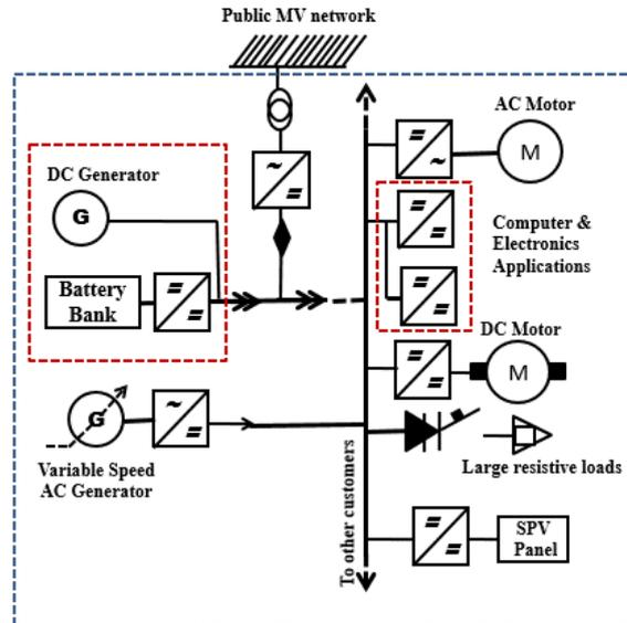
FIG 2:Schematic diagram of DC Micro-Grid.
