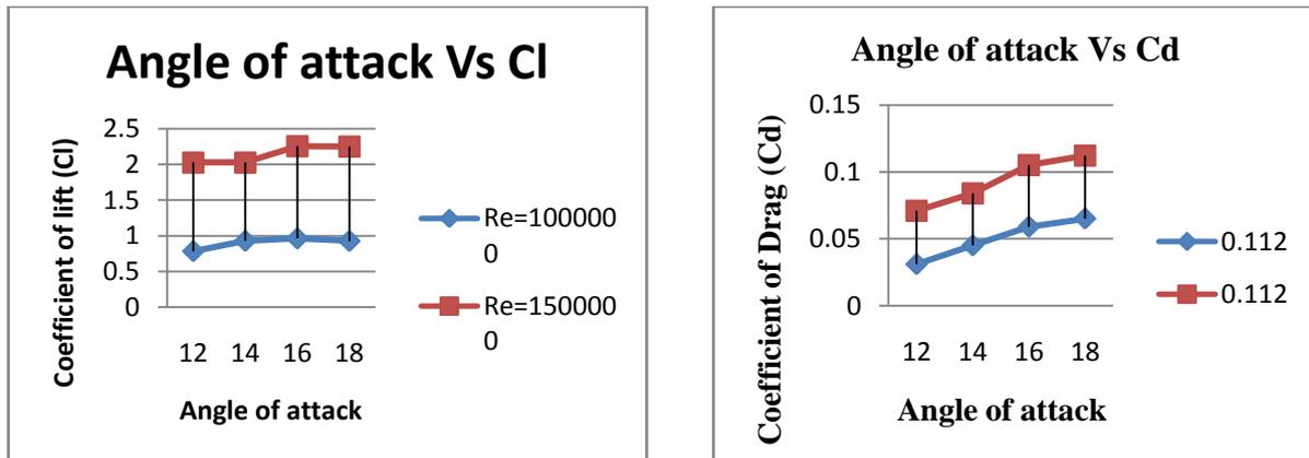
From above graph that as much as angle of attack is increased the coefficient of lift (Cl) is also increased hence lift is increase. But one condition comes when lift cannot be increased further and goes to reduced continuously. This reduction due to the generation of adverse pressure gradient at the trailing edge.
