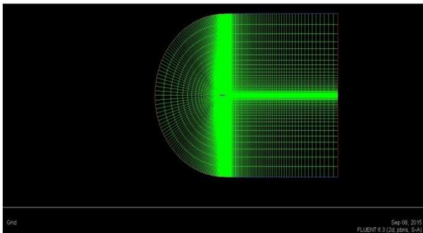
Figure - Upstream side of the airfoil C type
