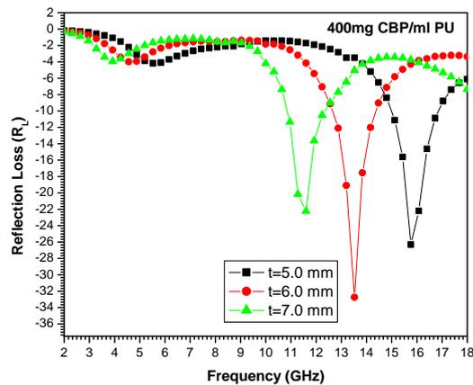
Fig. 4. Reflection loss ( $R_L$ , dB) vs. frequency (GHz) for  $t= 5, 6$  and  $7$  mm
