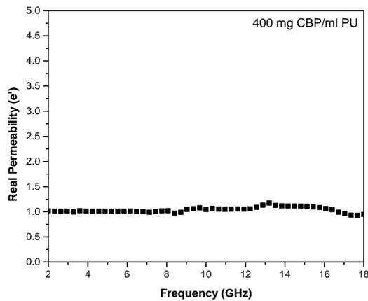
Fig. 3. Variation of Real permeability ( $\mu'$ ) with frequency (GHz) of CBP/PU Nano-composite
