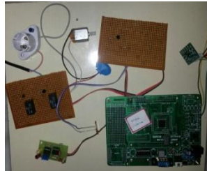
Fig 7: Integration of all sensors with ARM7
