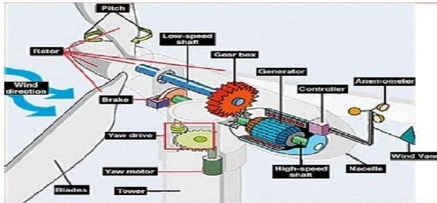
Figure 5: Internal Components of a Wind Turbine
