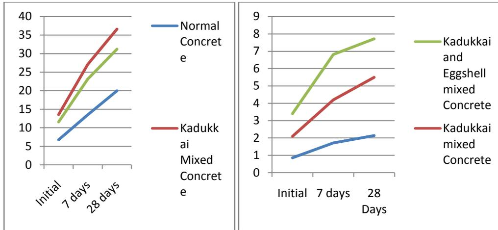
Fig. 4.1 compressive and tensile strength (normal concrete VsHerbocrete)
