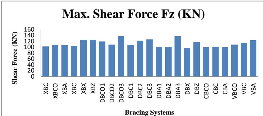
Fig 9. Maximum Shear Force Fz (KN) for different Bracing Systems
