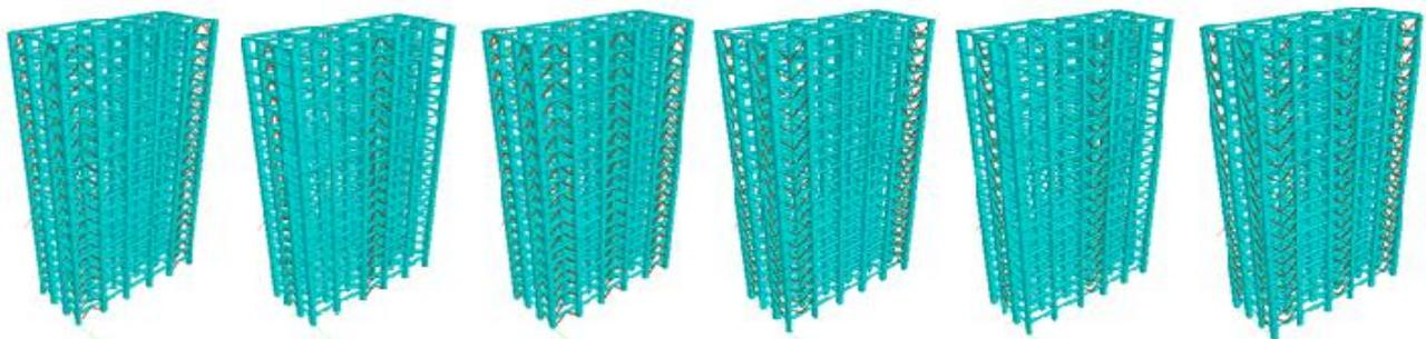
Fig 5: Chevron bracings and V bracings at corner,center and alternate locations
