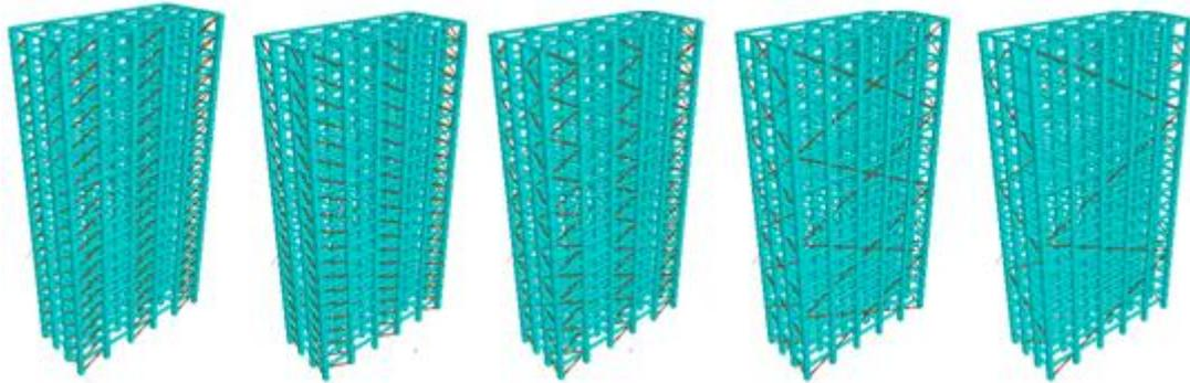
Fig 4: Different Locations of diagonal bracings
