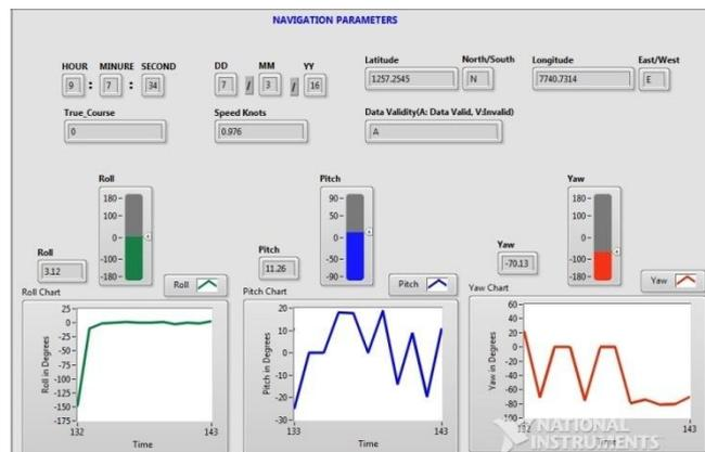
Figure 5-Displaying of hardware simulated navigation parameters in labview
