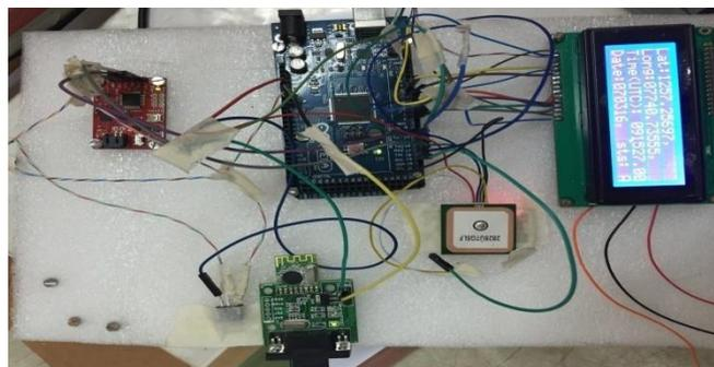
Figure 3- RF transceiver connected to ARDIUNO MEGA along with GPS-IMU system with LCD display
