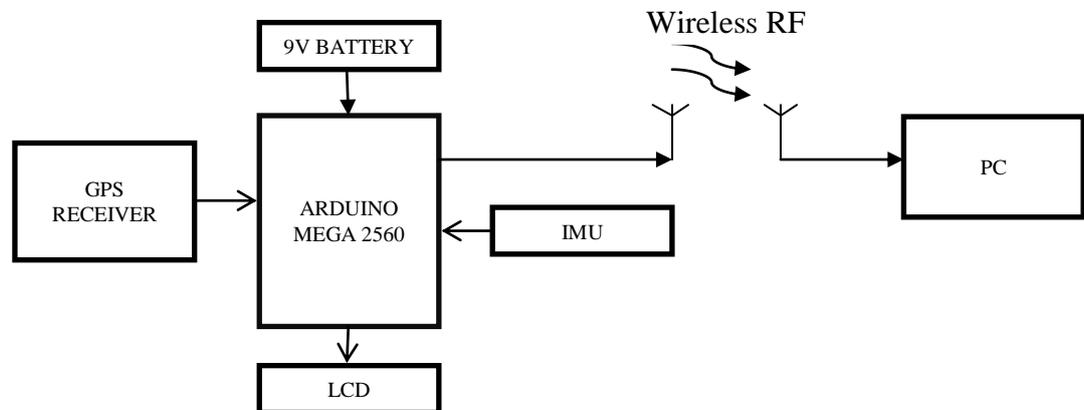
Figure 1- Block diagram of GPS/IMU system.
