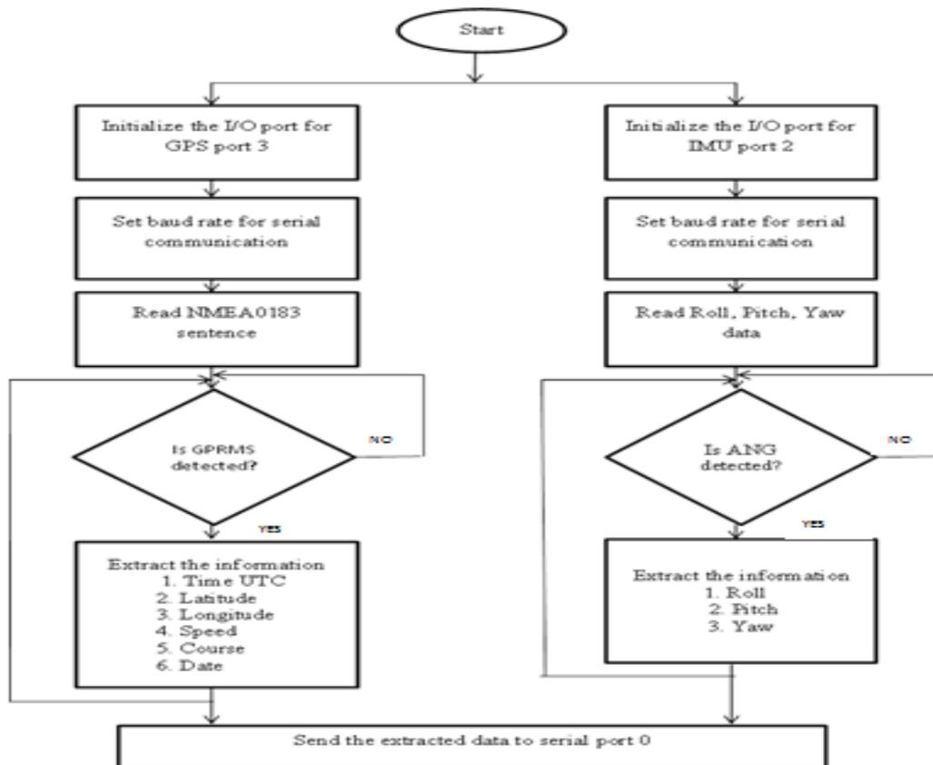
Figure 2-Flow of GPS/IMU system
