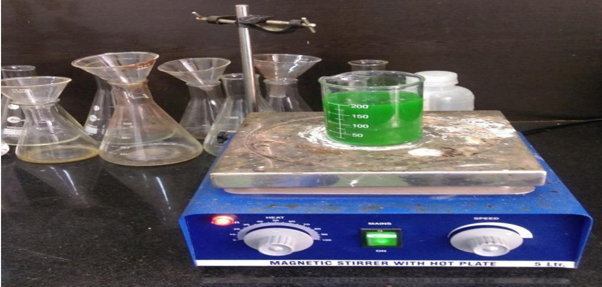
Fig No. 2 Preparation of nanofluid by magnetic stirrer
