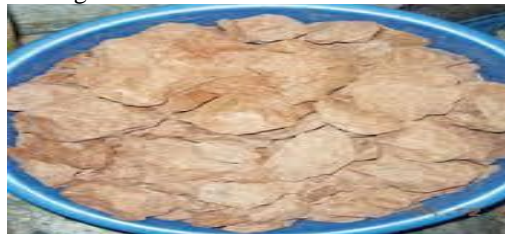
Fig. 2: The raw red mud (RM) used in the present
