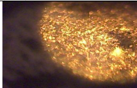
Plate 5. Micrograph of specimen subjected to heat input of 0.88kJ/mm using E7018 (X 400)
