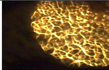
Plate 3. Micrograph of specimen subjected to heat input of 1.53kJ/mm using E7018 (X 400)
