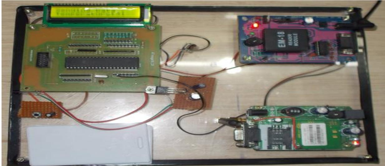
**Fig01: Integration of RFID and WSN (GSM Modem) with Data Cleaning Algorithm**
