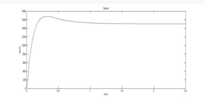
Fig 13.Phase currents using fuzzy controller Fig 14.Speed profile of the drive for fuzzy controller
