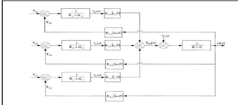
Fig 2. Transfer function model of BLDC motor
