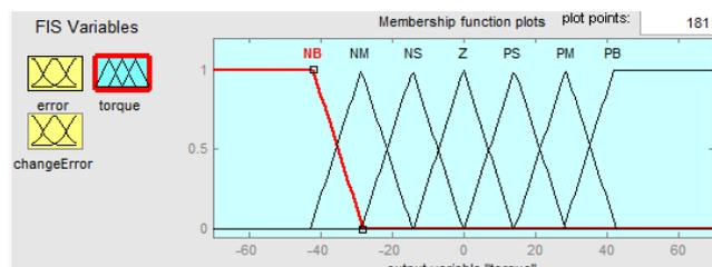
Fig 11.Membership function of reference torque
