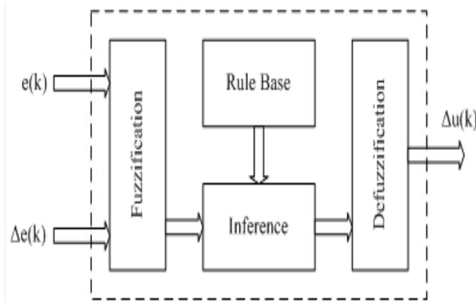
Fig 8 Structure of Fuzzy Logic Controller
