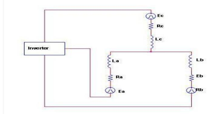
Fig 1. Equivalent circuit of BLDC motor
