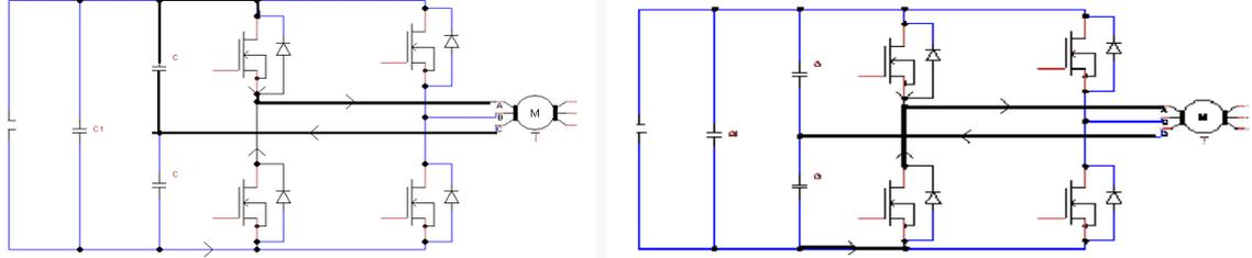
Fig 4.Sub operating modes 2a and 2b
