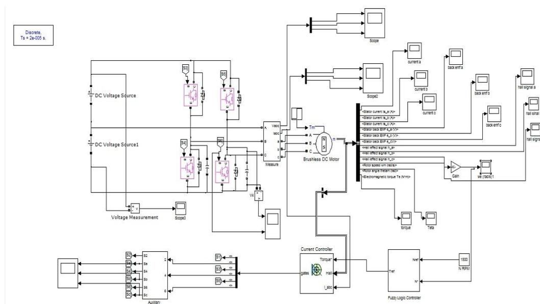
Fig 12 Simulink diagram of four-switch Inverter fed BLDC motor using fuzzy logic
