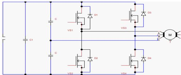
Fig 3. Four-switch three-phase inverter
