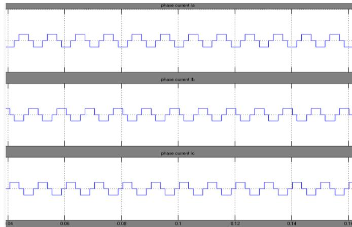
Fig 6. Phase current wave forms of Four-switch inverter fed BLDC motor
